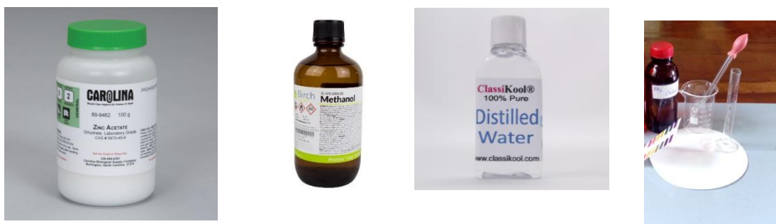
Figure 3 The materials used in synthesizing ZnO nanoparticles
