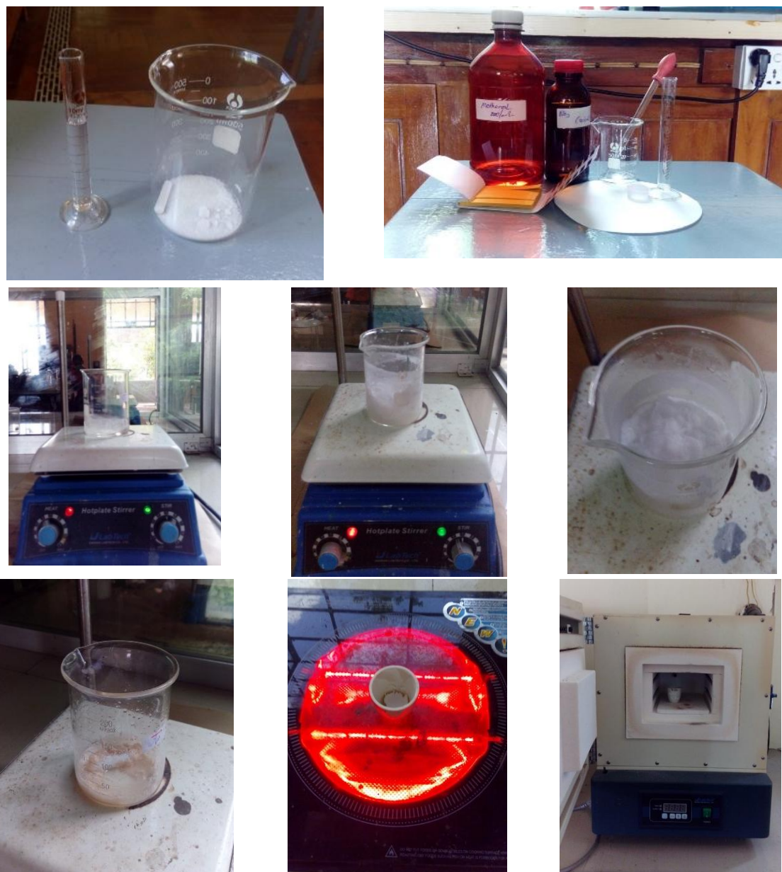
Figure 5 The procedures of ZnO nanoparticles
